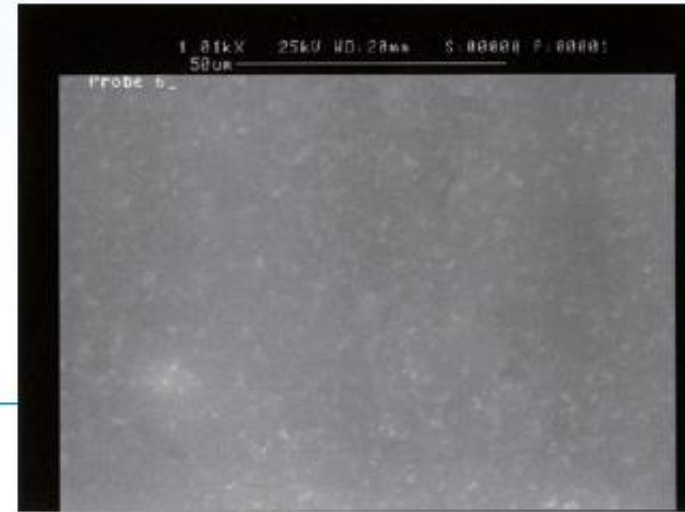
SEM* image of a standard ventricular catheter, typically of silicone
